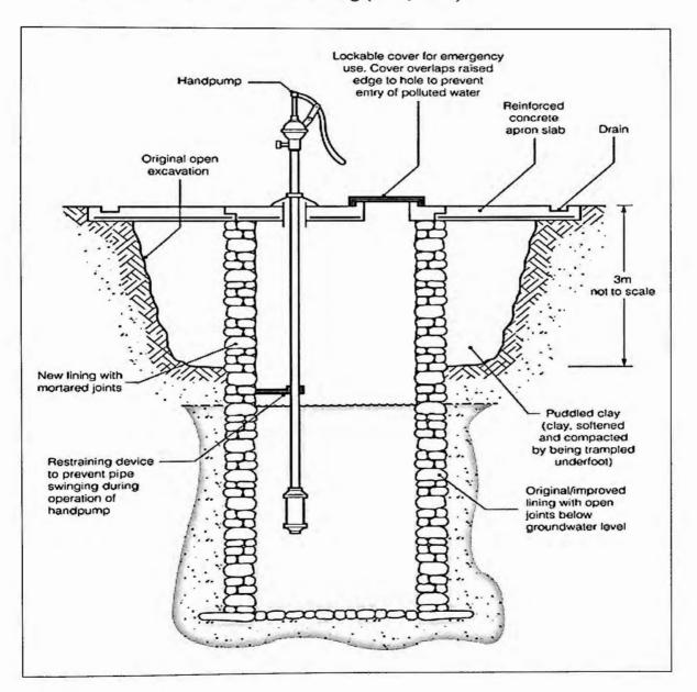
Figure 1.5: Diagram of a hand-dug well.
