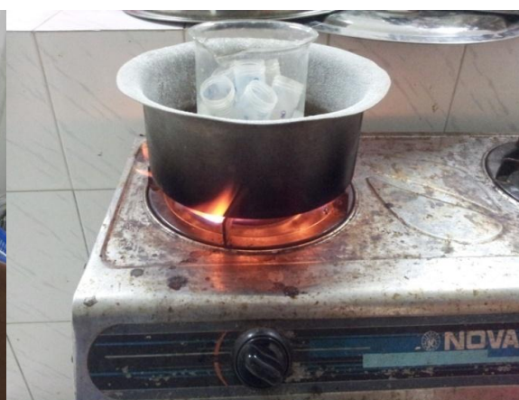
D: Test tube were placed in a boiling water bath
