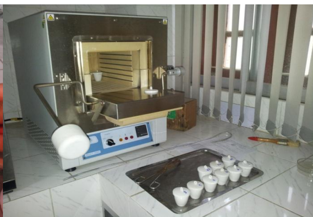
B: Crucible was placed in a muffle furnace
