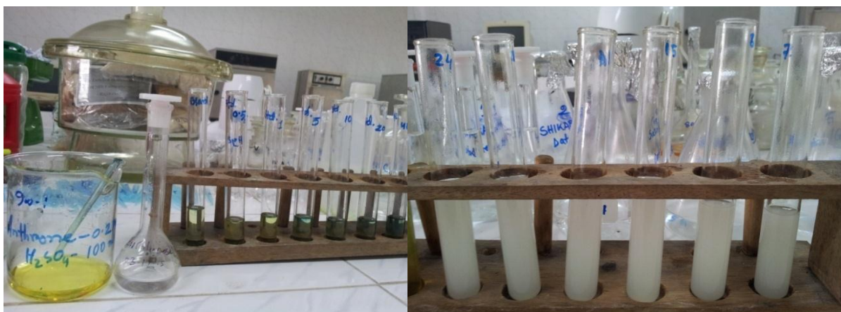
A: Anthrone reagent, standard glucose and blue-green sample solution
