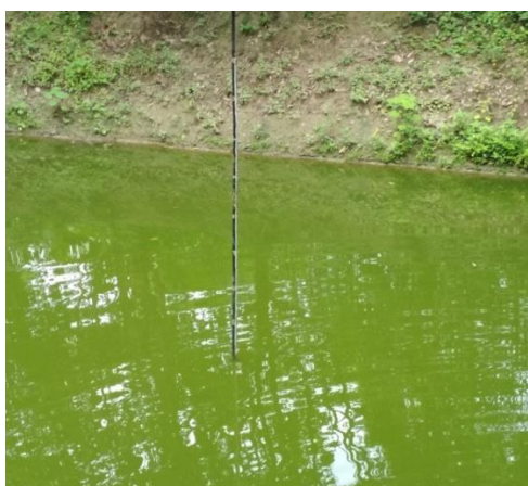
Figure 3.5: Water depth monitoring pipe
