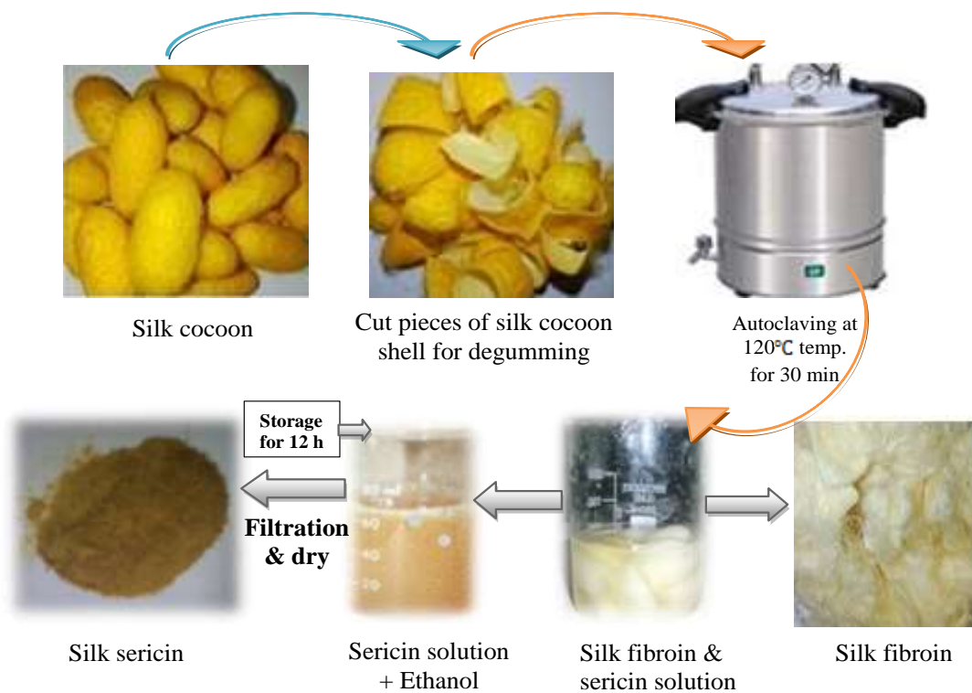
Figure 2.5: Schematic diagram of extraction process of sericin from silk cocoon
