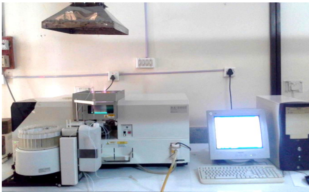
Figure 4.7 Atomic Absorption Spectrophotometer (Model No. AA-6800) coupled with an auto sampler (Model No.ASC-6100) used in present investigation.
