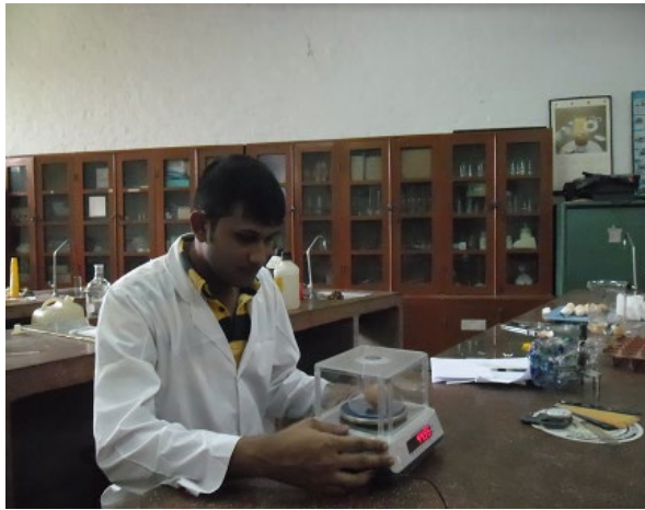
A Weighing of trial egg by a digital balance
