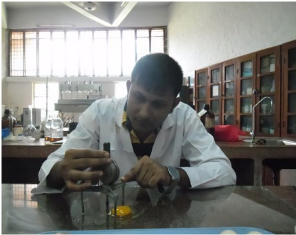
A Measuring albumen height by micrometer
