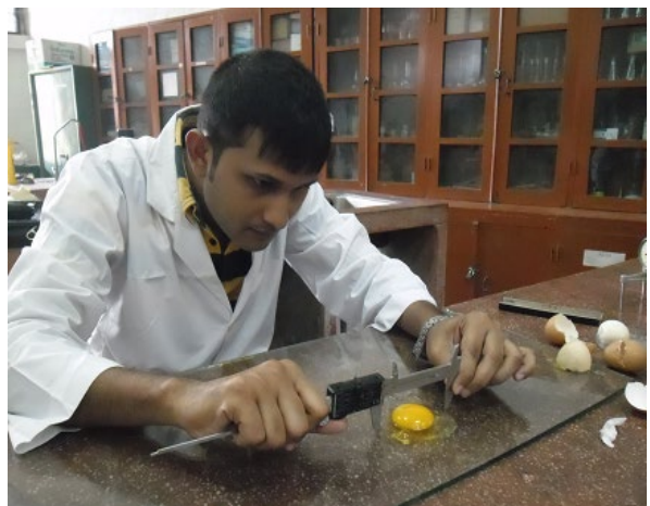
F Measuring albumen width by slide calipers
