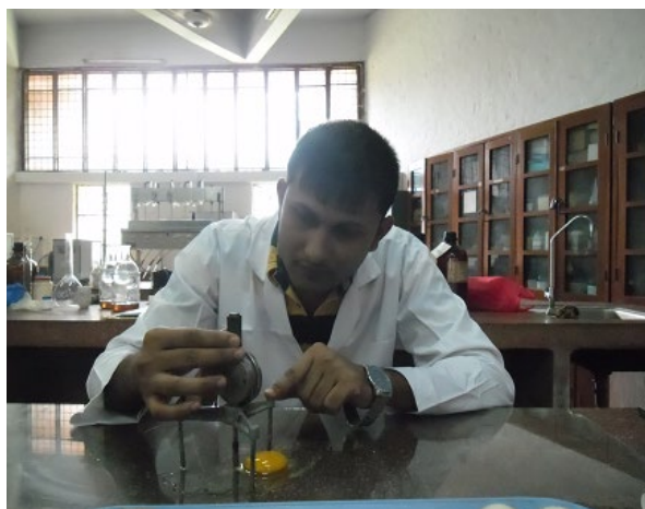
A Measuring albumen height by micrometer
