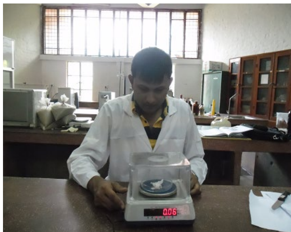
F Weighing shell membrane by digital balance
