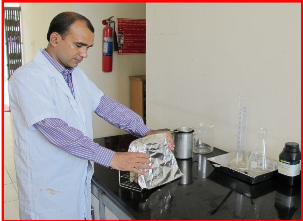
Plate 1c: Medium was poured into test tube and covered with foil paper
