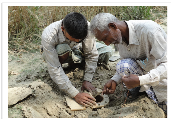
Photo-21: Static water level measurement in Sirajganj.
