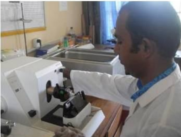
Figure C. Sectioning of the blocking liver tissue by microtome
