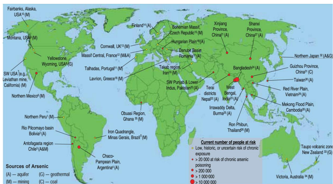
Figure 1.4 Worldwide distributions of arsenic contaminated regions, showing source of arsenic and numbers of people at risk of chronic exposure
