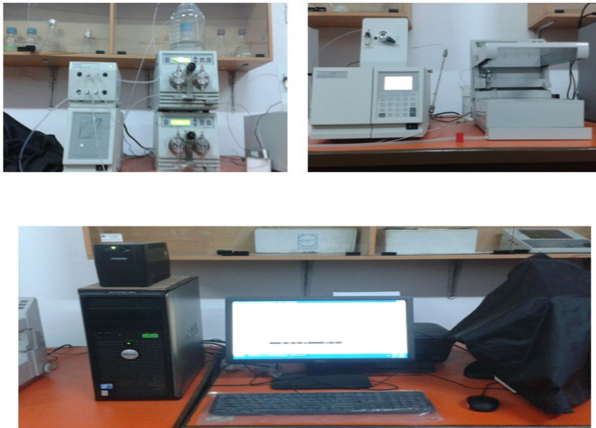
Plate 2.1: HPLC apparatus used to detect carbofuran concentration
