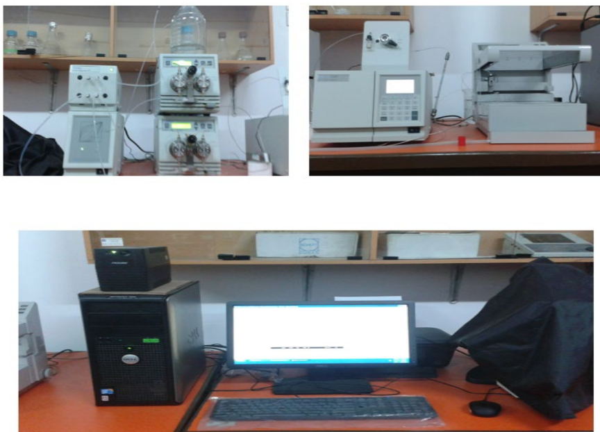
Plate 2.1: HPLC apparatus used to detect carbofuran concentration
