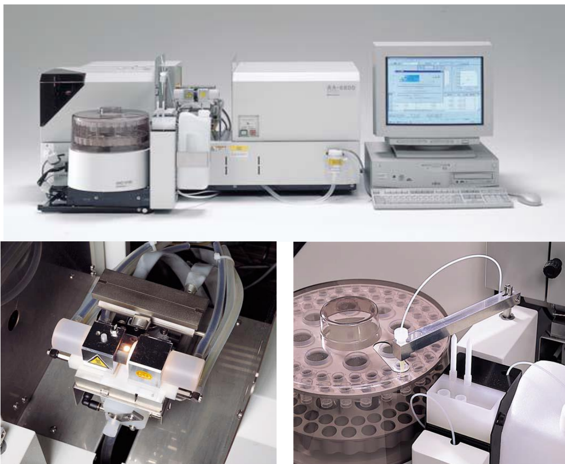
Figure 2.2 : Graphite Furnace - Atomic Absorption Spectroscopy (GF-AAS)
