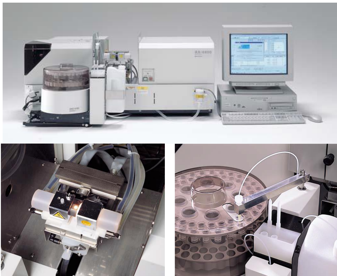
Figure 2.2 : Graphite Furnace - Atomic Absorption Spectroscopy (GF-AAS)
