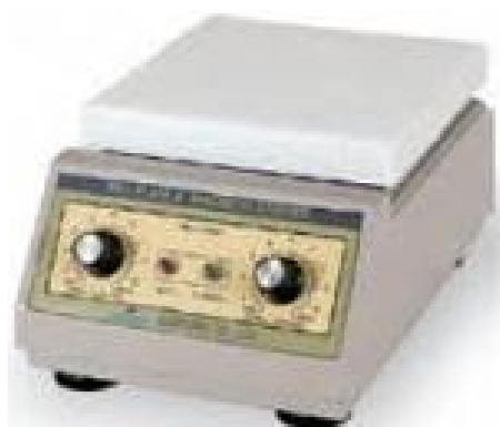
Hot plate and Magnetic stirrer
