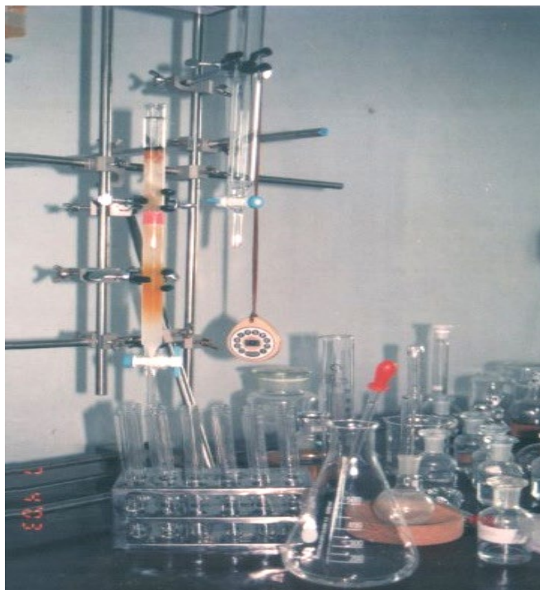
Plate16: Open column used in the experiment.
