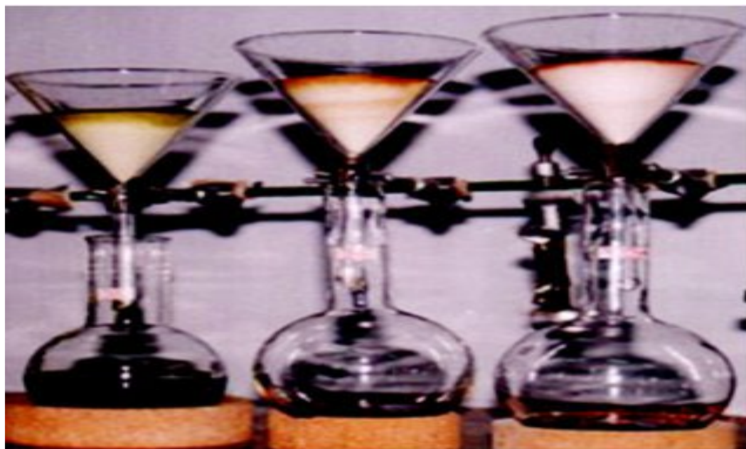
Plate 9: Filtration of chloroform and methanol extracts.
