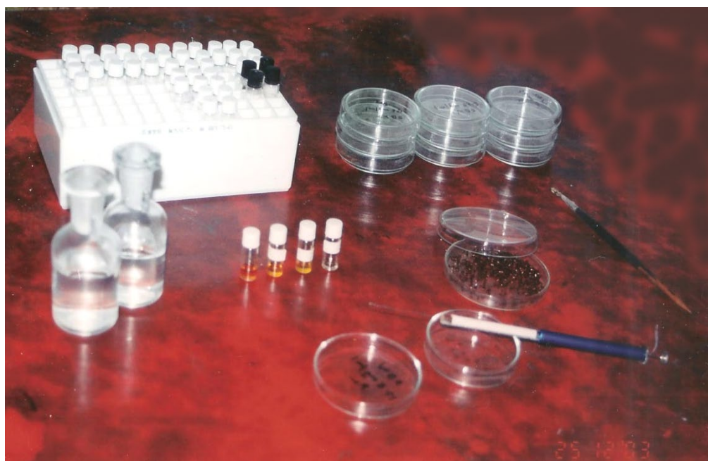
Plate12: Preparation of doses for surface film test
