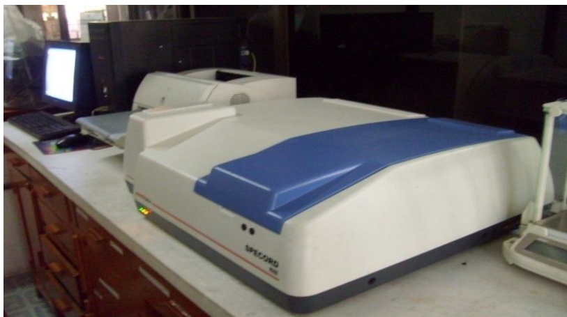
Figure-2.3.1: Double beam Analykjena UV/Visible spectrophotometer (Model 205, Germany)
