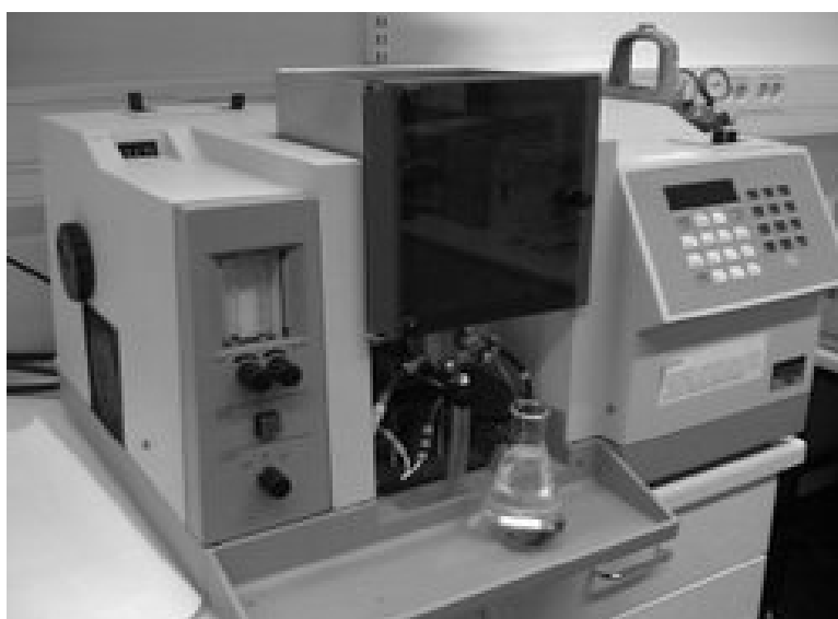
FIGURE 2.2: Atomic Absorption Spectrophotometer (AAS) used in this study
