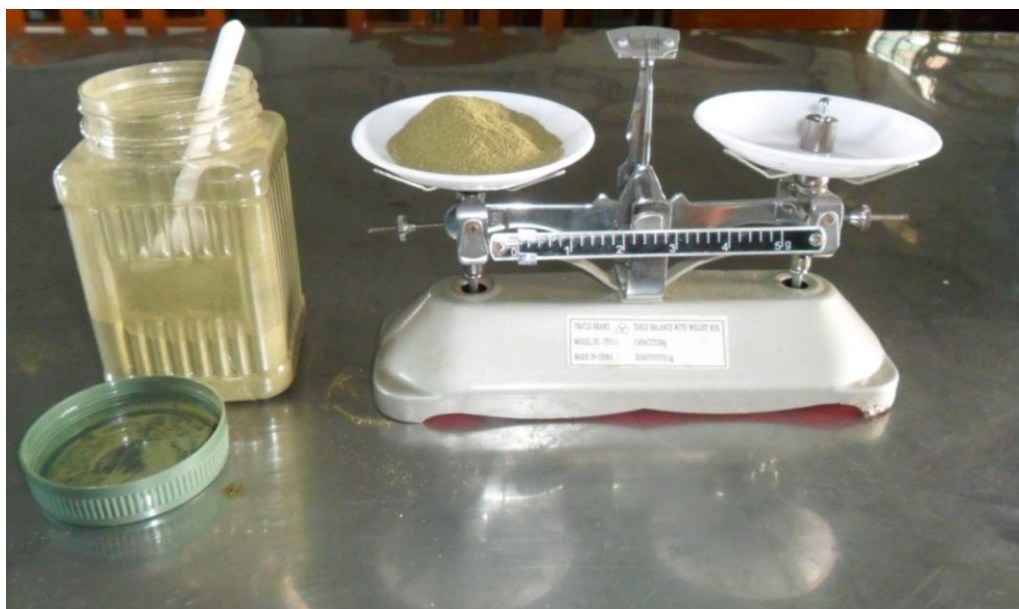
Plate 30. Measurement of plant powder with balance and weight box
