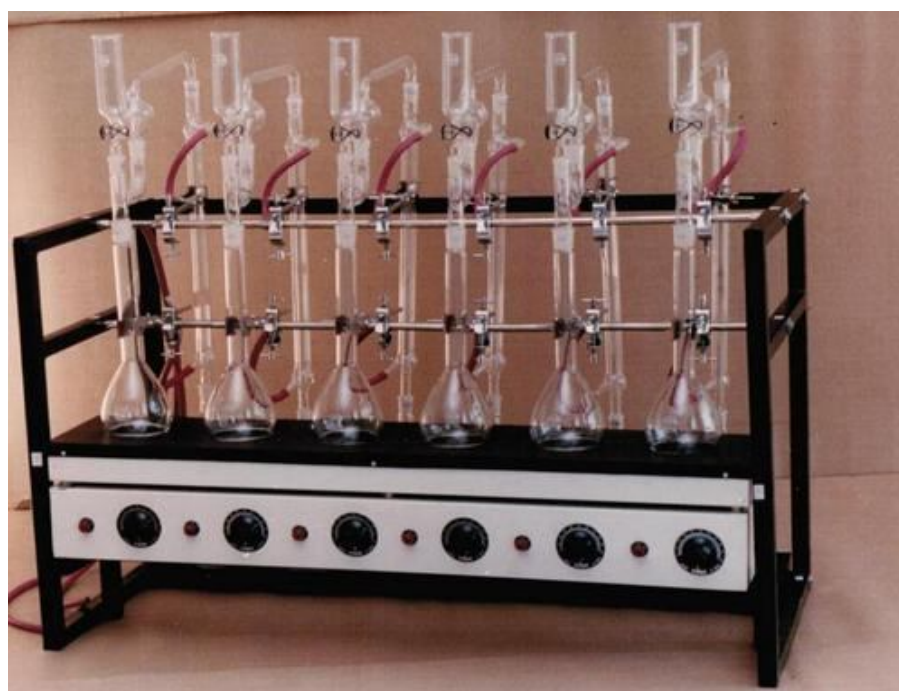
Figure 2.8: A view of the protein analysis of the sample under present study (Distillation Process)
