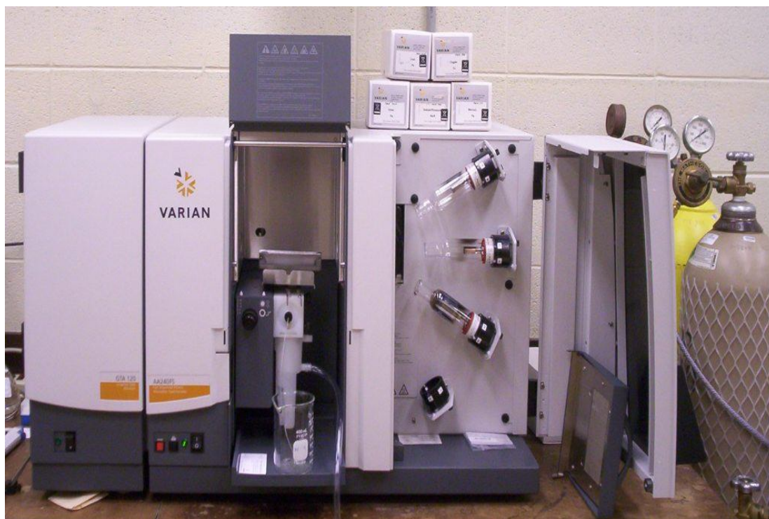
Figure 2.9: Atomic absorption spectrophotometer. Model AAS 240 VARIAN, Australia.
