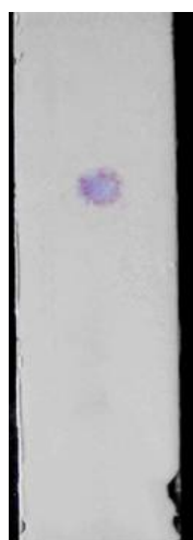
Figure 2.4 Purity of compound-4 on TLC plate using the solvent system of n-hexane and ethyl acetate (19 : 1)
