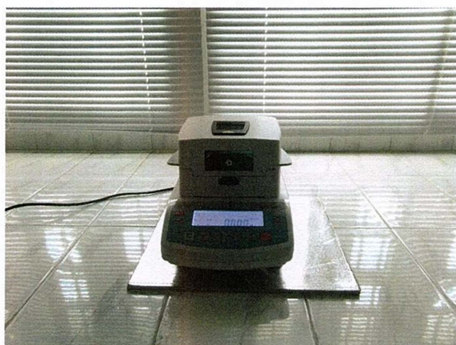
Automatic moisture analyzer
