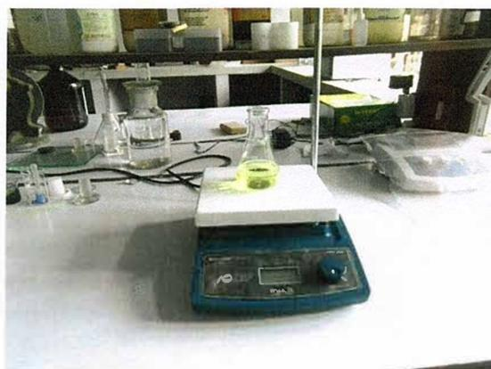
Magnetic stirrer with heating (Phosphorous digestion)
