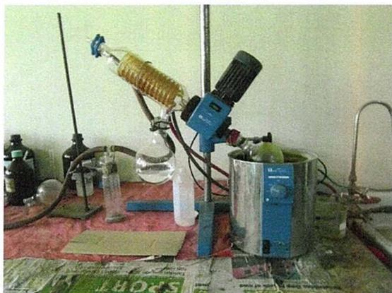
Rotary evaporator with vacuum pump (Fat)
