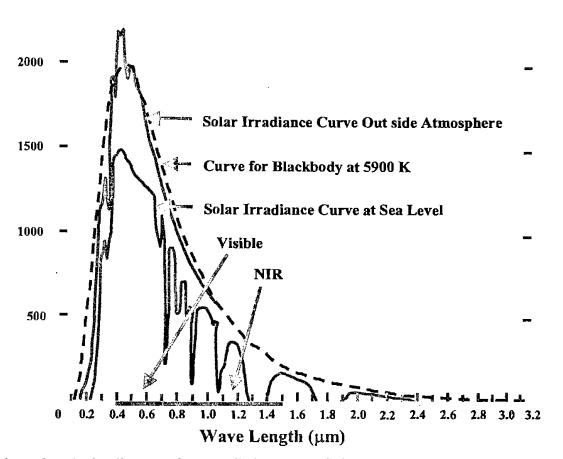
Figure 2.1: A plot diagram of solar radiative energy derived with the help of Planck's law.
