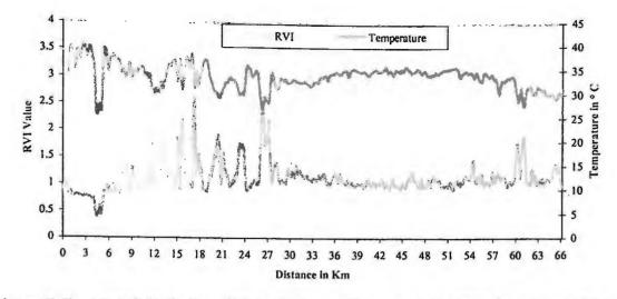
Figure 7.5b: Spatial Variation of Surface Temperature and Satellite Based RVI Value as derived from Landsat TM image dated October 20, 1990.
