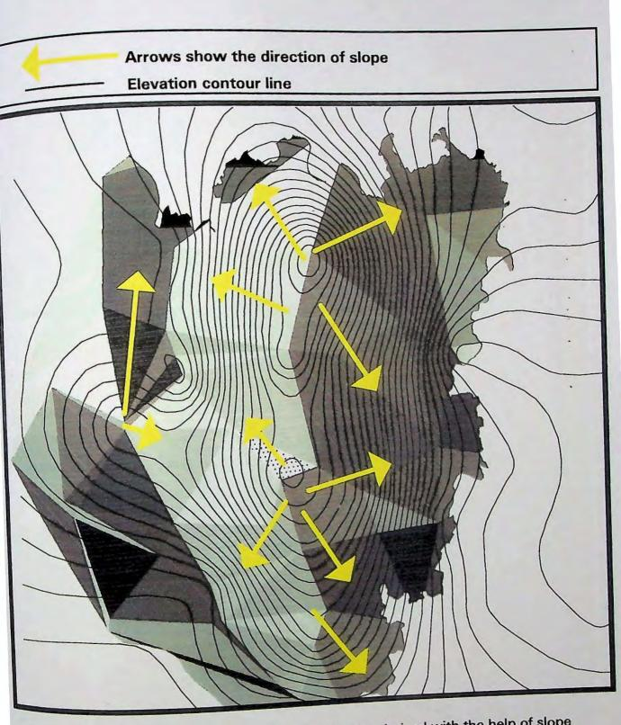
Figure 10.5: Shaded relief of surface water redistribution derived with the help of slope aspect image.
