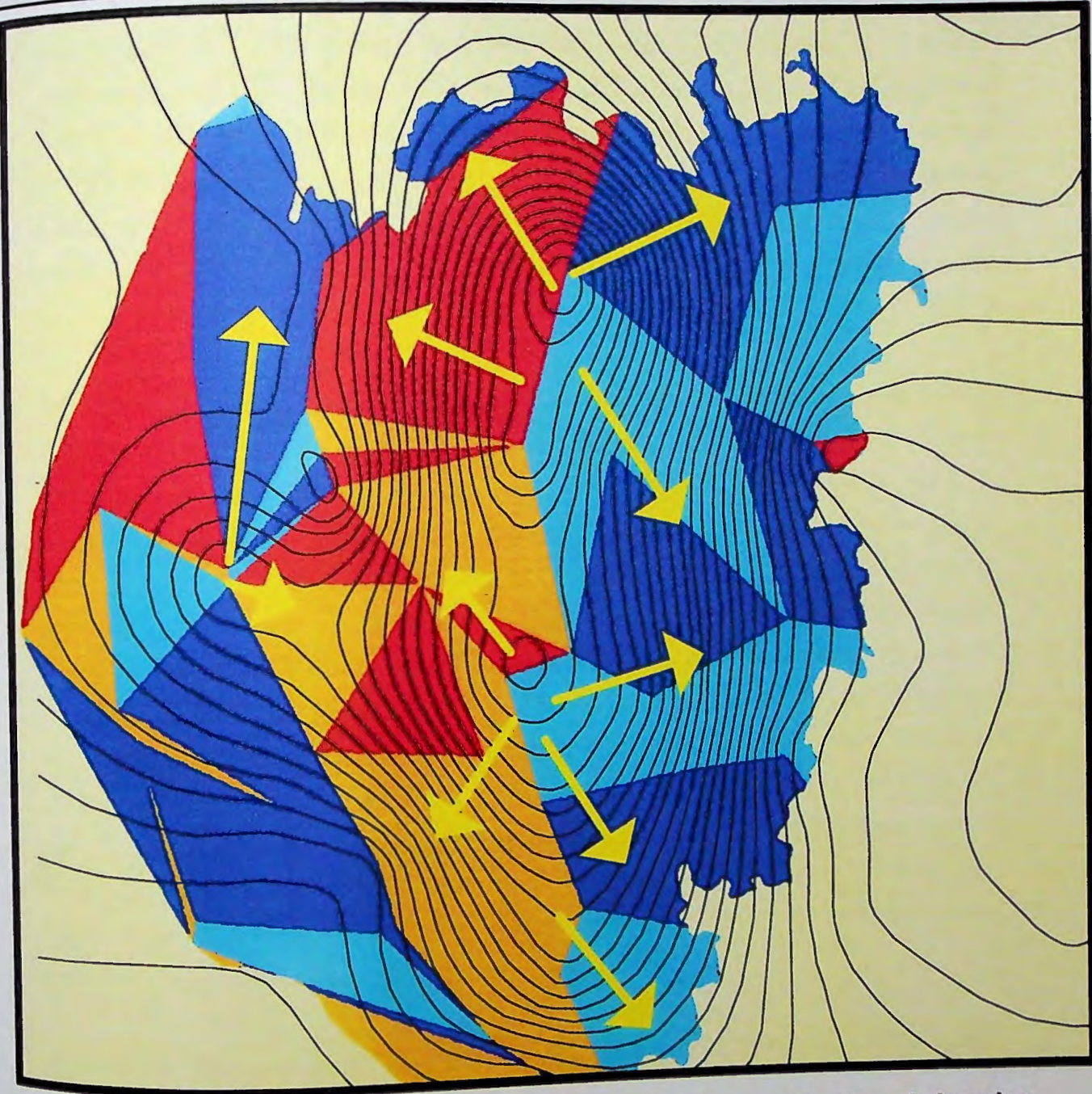
Figure 10.4: Slope aspect of study area as derived from the combination of elevation data and Landsat TM image.
