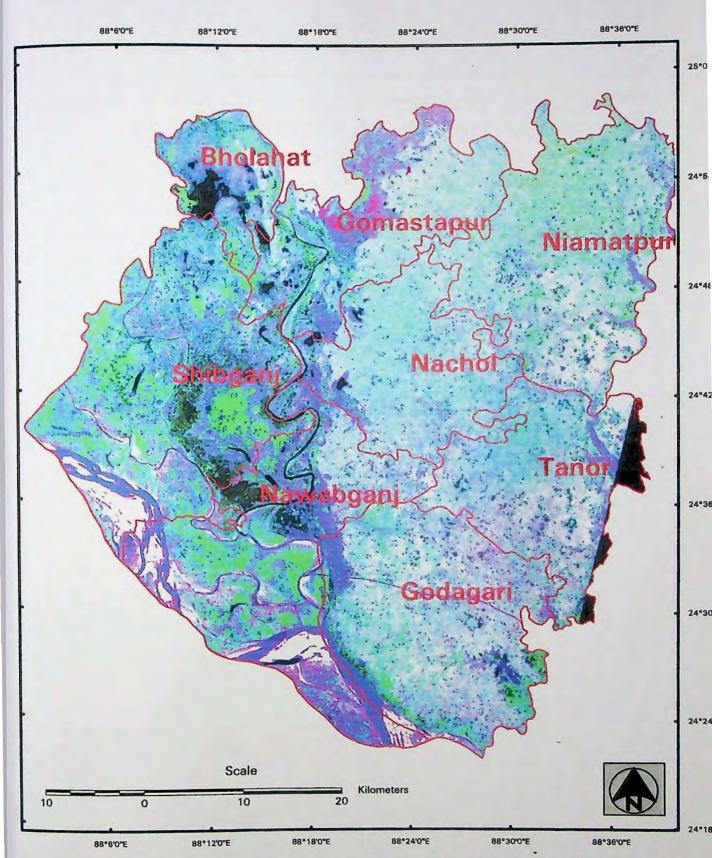
Figure 7.1c: Spectral colour composite of Landsat TM (February 09, 1991) of Barind Tract and flood plain areas, in the north-western part of Bangladesh. The composite is composed of Bands 5, 4 and 3 (red, green and blue).
