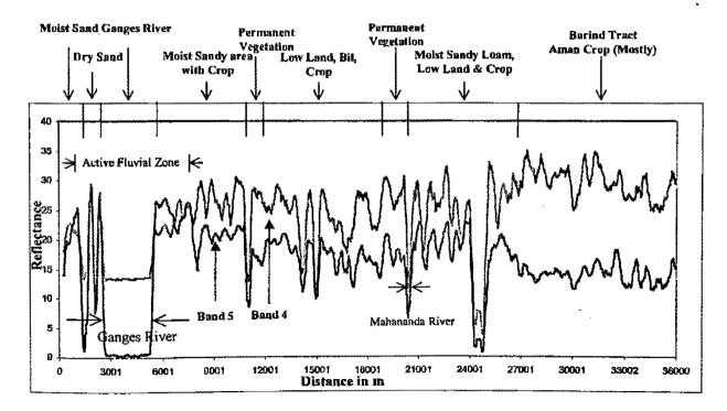
Figure 6.2b: Change of surface types due to seasonal as well as climatic change with respect to the surface types in summer detected by Landsat TM satellite data.
