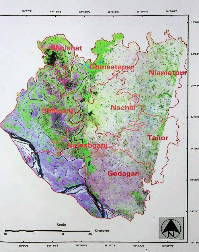
gure 7.1a: Spectral colour composite of Landsat TM (April 11 1990) of Barind Tract and flood pl reas, in the north-western part of Bangladesh. The composite is composed of Bands 5,4 and 3 ed, green and blue). 39
