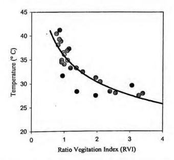
Figure 7.6: Dependency of satellite based surface temperature on the satellite based vegetation index.
