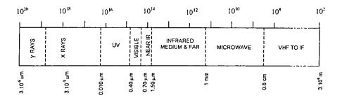
Figure 3.1: The Electromagnetic spectrum with wavelength (adapted from Parker and wolf 1965, Estes and Senger 1974).
