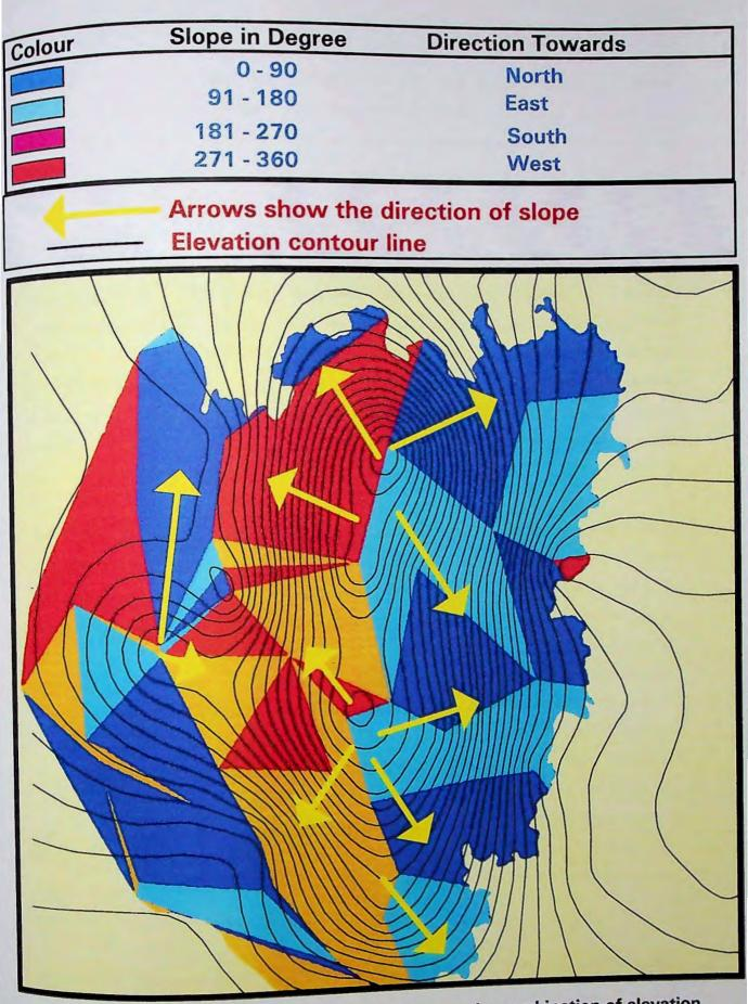
Figure 10.4: Slope aspect of study area as derived from the combination of elevation data and Landsat TM image. 92
