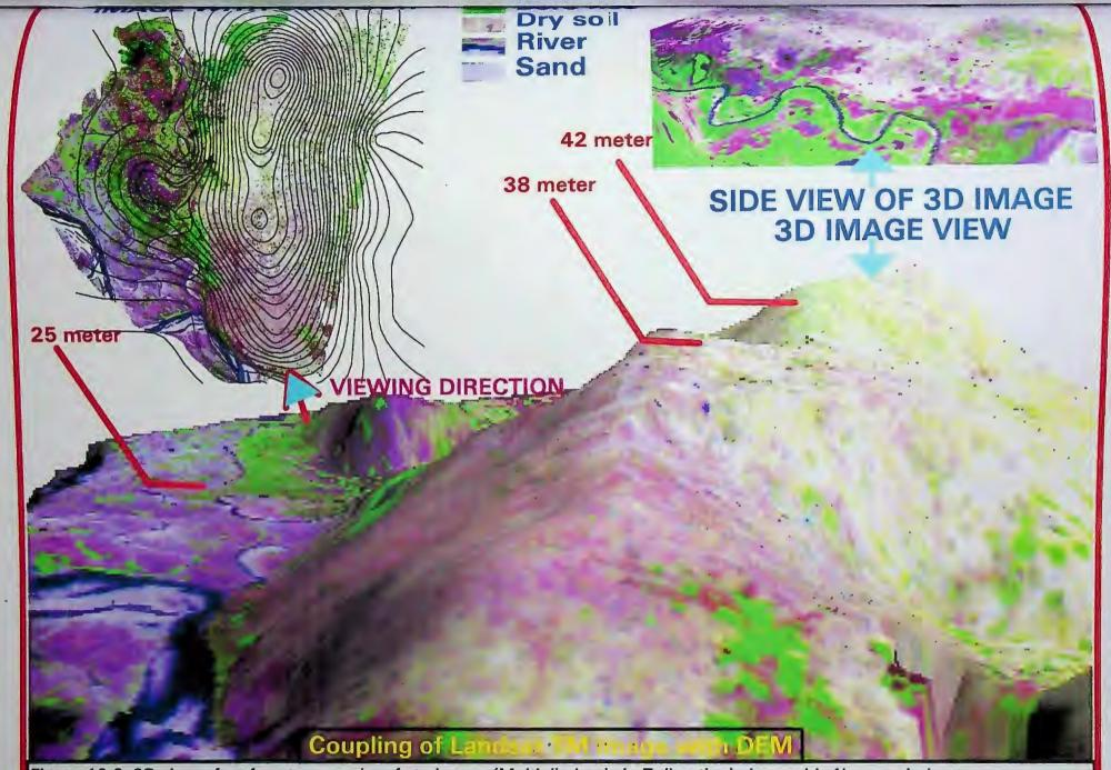
Figure 10.6: 3D view of surface topography of study area (Multiplied only in Z direction) along with 1km resolution DEM contour map. 95
