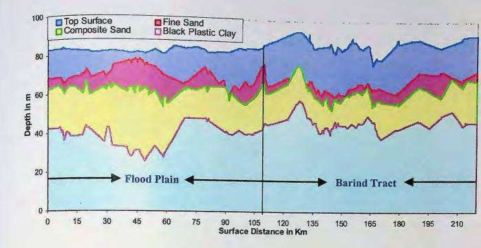
Figure 11.2: Compositional arrangement with varying thickness of sub-surface formation for both
