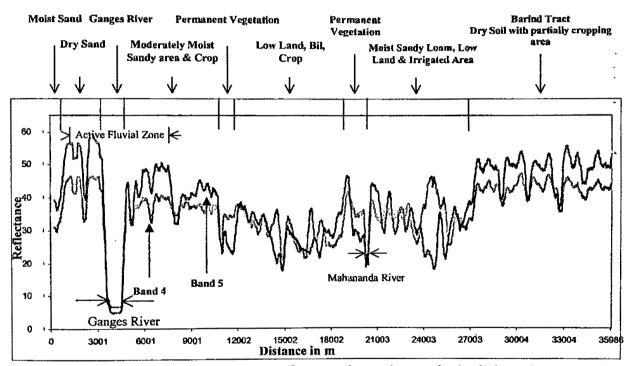
Figure 6.2a: Types of surface along a profile over the study area in April 1990 (Dry season) identified by Landsat TM satellite data.
