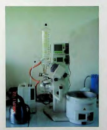
Plate 15 : Evaporation of mixed solvent from extraction by a Vaccum Rotary Evaporator (Rota vapor R-215)
