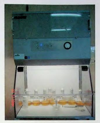
Plate 16 : Laminar Air Flow Unit (Model No. NU- 126-300E)
