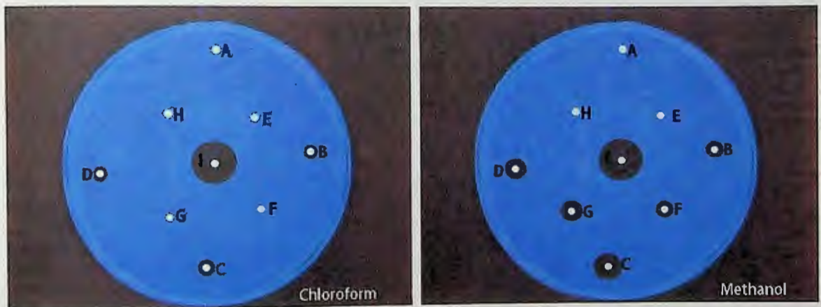
Plate 23 : Effect of chloroform and methanolic extracts from different parts of tit begoon and kumarilata and standard Ciprofloxacin (30 \mu g/disc) against Staphylococcus aureus
