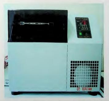
Plate 13 : Shaking Incubator ( DK-SI 010 )
